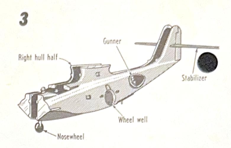
Apply glue to bumps which align stabilizer and around edges of right hull half. Then carefully slip right half of hull over stabilizer as shown above and press together. Bind with rubber bands if necessary to hold hull halves tightly together. Remove rubber bands after glue dries.
