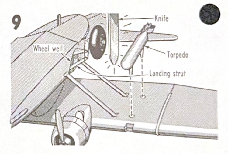
Glue landing struts into holes in wheel well. Then slip rubber wheels onto axles. Flare end of axles with the heated blade of an old knife as shown. If desired, the wheels can be glued into wheel wells in retracted position. Glue torpedoes to wing.
