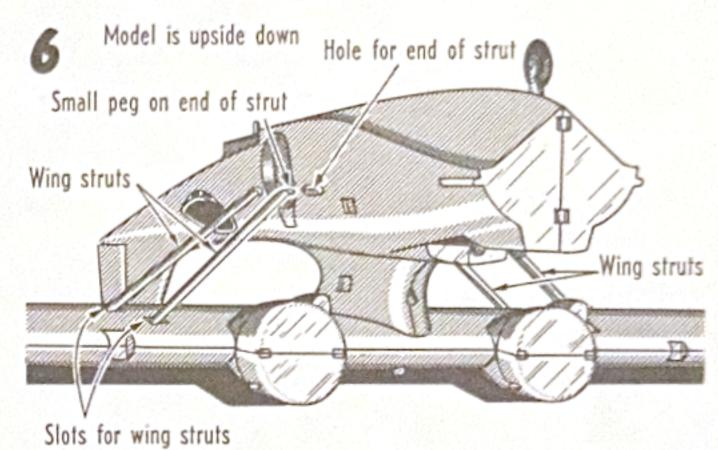
Lay model upside down and install four wing struts. Notice that each strut has a small peg at one end. This peg fits into hole in hull and other end fits into square slot in wing. Slip strut into slot in wing first and then fit peg into hole in hull.
