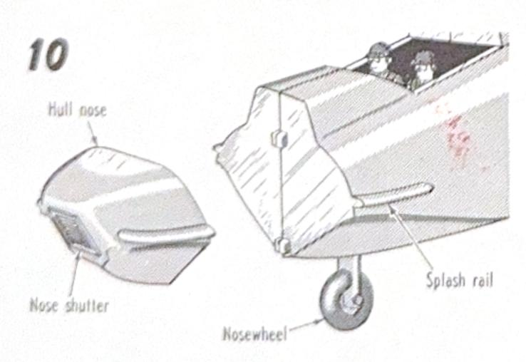
Glue hull nose in place on front of hull. If you are making your model with landing gear retracted as though in flight, the nosewheel and rear skid can be cut away with a small saw and then carefully trimmed clean.
