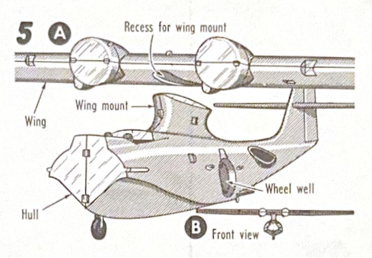
(A) Glue wing to hull assembly. Top of wing mount fits into recess in bottom of wing for correct location. (B) Push wing down firmly onto wing mount so one wing tip will not be lower than the other when viewed from the front.
