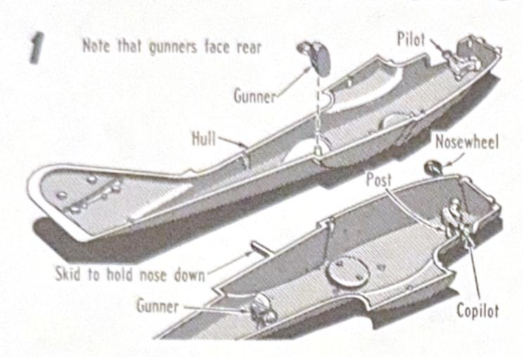
Glue pilots and gunners onto posts on inside of hull, making certain they are pushed on all the way. The small skid on bottom of hull is provided to keep the nosewheel of the model on the ground so balance weights are not needed.
