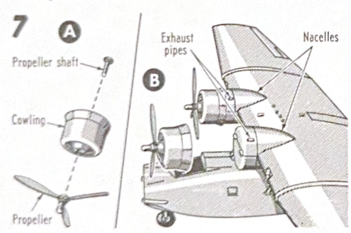
(A) Insert propeller shaft through hole in cowling from the rear. Apply a bit of glue into hole in propeller and press shaft into propeller. Prop should spin freely, (B) Glue cowlings in place on front of nacelles.
