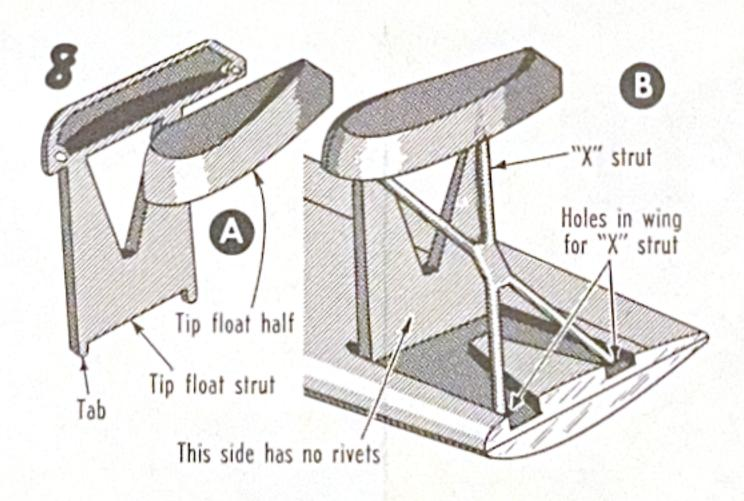
(A) Glue tip float halves to tip float struts. (B) Turn model upside down and glue tip float strut to wing in position shown. Then glue "X" strut in place. If desired the tip floats can be glued to the ends of wing in retracted position.
