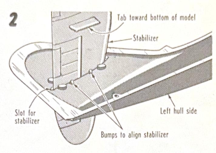
Before gluing hull halves together, carefully slip stabilizer into slot in tail of left hull side as shown above. Notice that tab on stabilizer should be toward bottom of model. Glue this tab against small bumps inside which align the stabilizer.
