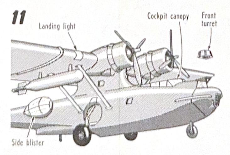
Glue front turret, cockpit canopy and side blisters to hull. Also glue landing lights into recesses in leading edge of wing. Use glue sparingly so it does not squeeze out onto outer surfaces.
