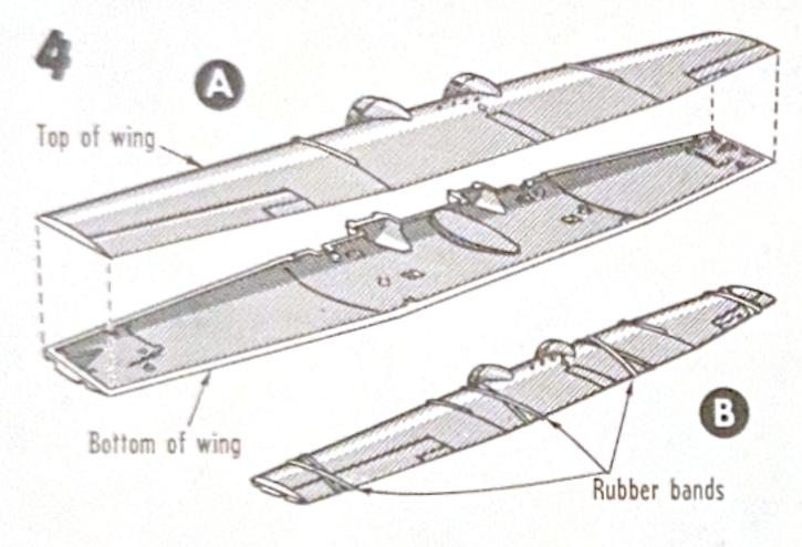
(A) Glue top of wing to bottom of wing. Work quickly and carefully. Do not get glue on outside edges as it will spoil the finish on the model. (B) Hold top and bottom together with rubber bands if necessary while glue dries to prevent gaps between the pieces.
