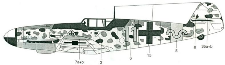
Bf109G-2, W. Nr. 13670, 9./JG 52, flown by Oblt. Hermann Graf, Galjagewskaja, Russia, September, 1942. Camouflage is RLM 74 Graugrün & RLM 75 Grauviolett over RLM 76 Lichtblau. Lower cowl, fuselage band, and lower wing tips are RLM 04 Yellow. Spinner is RLM 70 Dunkelgrün and white, spinner backing plate is RLM 70. Fuselage mottling appears to be RLM 74 and 75. Note: use templates provided for painting interior part of fuselage crosses RLM 74.
