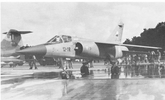
Mirage F.1c No. 67 '12-YR' of E.C. 1/12, Armée de l'Air, from Cambrai; at this time, the unit had received the first two or three of these machines, main equipment still being the Super Mysteres (see Set 46). As with French Jaguars, the Mirage F.1's are often seen in clean configuration (i.e. no stores underwing), so this can be optional on a model. Note the fixed spotlight in the port intake flank, this being used to illuminate certain airborne intercepts following radar lock-ons at night. Photo: RLW.
