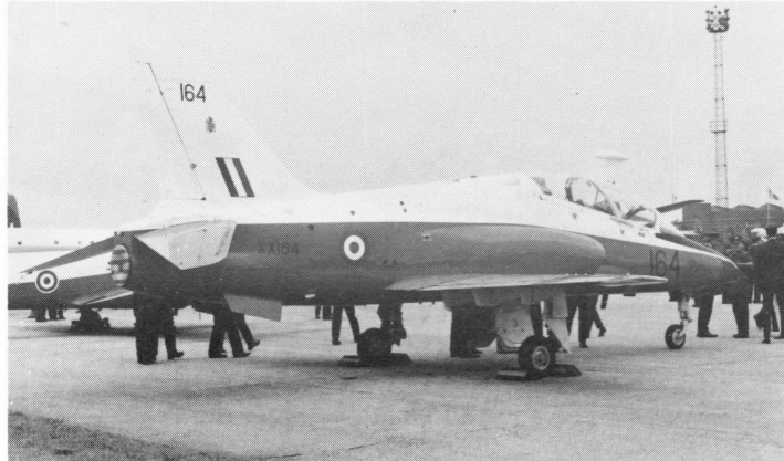
XX164 of the CFS again, this time a month later in the static park at the Finningley Review and in spotless finish. Apart from the wing fences, the other prominent addition to production Hawks is the pair of angular ventral fins fixed to the fuselage immediately outboard of the air brake. Again note the attitude of the tailplane when at rest, and the inboard main under-carriage doors hanging down. The CFS and 4 FTS Hawks are operated as a single unit at Valley. Photo: RLW.
