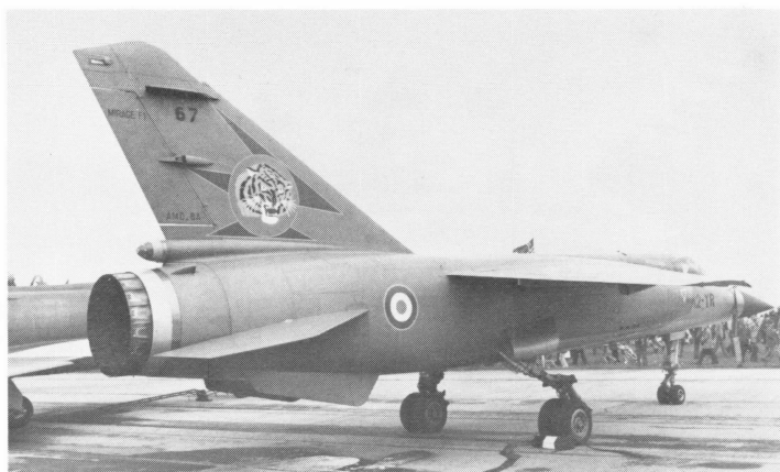
Rear view of '12-YR' showing the very attractive emblem used by E.C. 1/12, the tigers head being the emblem of SPA162, the hornet on the port side the emblem of SPA89; in fact the Mirage F.1's carry some of the most colourful unit artwork yet seen on French military aircraft. Note lack of fin-mounted ECM pods seen on some machines, and the angle of the tailplane when the machine is 'at rest'; all-flying tailplanes on most types are rarely horizontal when on the ground. Photo: RLW.
