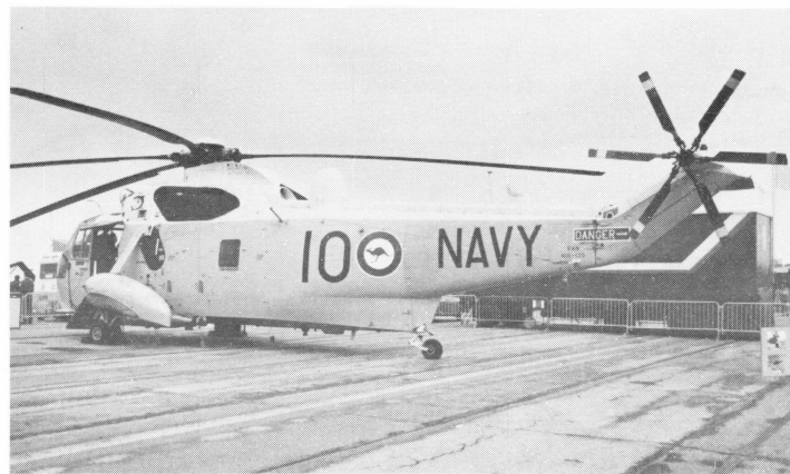
N16-125 again, showing its port side markings, also earlier in the display before the nose 'zaps' were added. Note the six-blade tail rotor fitted to the later Sea Kings; the additional blade is easily made – aligning them may prove slightly more interesting! The port cabin window of the kit needs to be located further back; fill old opening, and fit new square window to new opening. Note also the dorsal radome and blade aerial. Photo: RLW.
