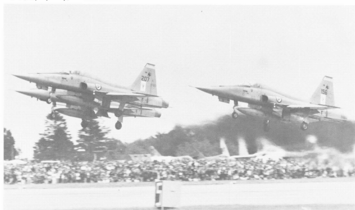
Three of 'The Jokers' F-5's getting airborne for their display at the Air Tattoo, led by 207. The varying camouflage of the belly fuel tanks is apparent; note that there is a thin pipe which runs from the top of this tank into the belly of the aircraft, shown on the drawings, and is probably part of the smoke apparatus for the team's displays. On your model, the lacquered silver appearance of the paintwork could be obtained by mixing silver with a little light grey and matt polyurethane varnish. Photo: RLW.
