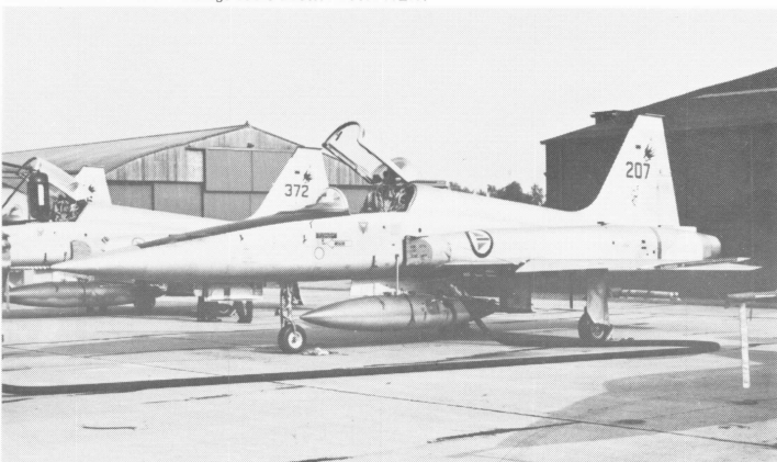
F-5A(G) 207 of 'The Jokers' aerobatic team from No. 336 Sqn., Royal Norwegian Air Force, based at Rygge. Note that wingtip tanks were not fitted at the Air Tattoo, manoeuvrability being improved by fitting Sidewinder rails instead of tanks. Belly tanks were fitted, and on the aircraft at Greenham Common were camouflaged matt (NATO) dark grey on top, with matt aluminized-polyurethane (silver) underneath. Note also the drooped wing leading edge slats. Photo: B. Pickering, MAP.
