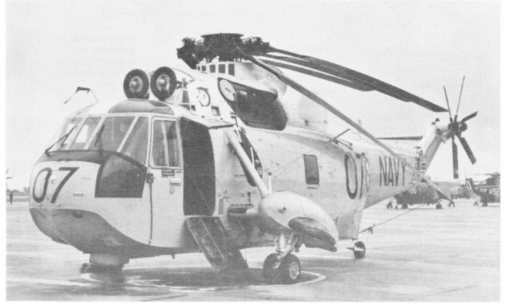
N16-118 '07', the third Sea King option on the decals, also at Yeovilton on 28th June. If amending the tail rotor proves too easy, folded main blades will exercise your skills a little more. Note the opened crew entry doors, the lower one with steps on its inside face; also the aerial wire to port only, with the gloss white aerial masts to the undercarriage sponson and fuselage. Sea Kings have a mass of minor lumps and bumps etc. which can be added to Airfix's excellent kit. Photo: P.J. Cooper.
