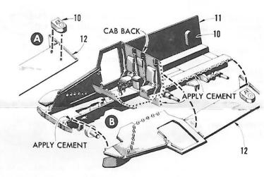
(A) Cement an ammunition case 10 to each body side 11 and 12 near rear. Pins on body sides fit into holes in cases. (B) Attach body sides as indicated in sketch. Make sure sides are pressed tightly in place.
