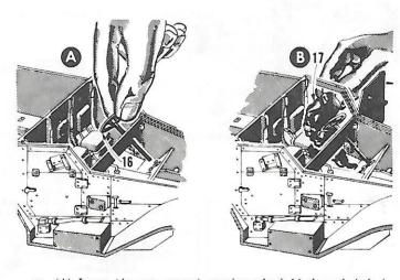
**6** (A) Insert (do not cement) steering wheel 16 through hole in dashboard so end of steering column fits into slot in floorboard.
