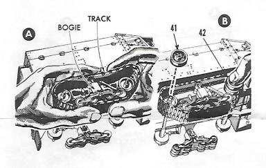
15 (A) Slip tracks over bogies and then around inner driver and idler wheels. (B) When track is in place, press outer idler 41 and driver 42 wheels onto axles past retaining buttons so wheels turn freely.
