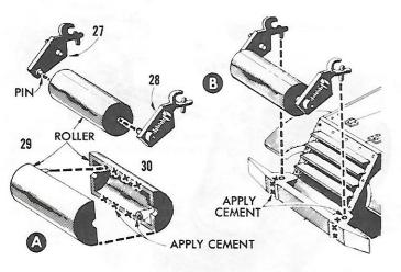
11 (A) Cement roller halves 29 and 30 together. Do not get cement on ends or roller will not spin on roller brackets. (B) Slip pins on brackets 27 and 28 into holes in roller. Do not cement. Apply cement to bumper as shown by X's. Hold roller and brackets together between thumb and finger and attach unit to bumper.
