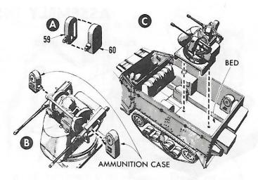
**20** (A) Cement ammunition case halves 59 and 60 together. (B) Apply cement into slots in machine guns and attach the ammunition cases as shown. (C) Apply cement to bottom edges of turret mount fit into holes in bed. Cement radio operator to left gas tank as shown in main exploded drawing.
