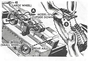
14 (A) Snap inner idler 39 and driver 40 wheel halves over axles. Small wheels go on rear axle. (B) Join track by holding ends as shown. Bend end of track into a "V" with right hand and insert into open end of track.
