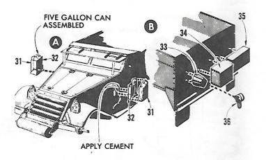
12 (A) Cement five gallon can halves 31 and 32 together and attach them to right and left body sides. Pins on cans fit into holes in body sides. (B) Cement bucket 33, ration box 34, and blanket box 35 to body back. Apply cement into slot in body back and press short tab of hook 36 into slot.
