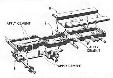
2 Apply cement to frame 7 and front axle unit 6 as indicated on drawing. Attach front axle unit so that two lineup holes on bar fit over lineup pins on frame. Also, front axle fits into notches on frame. Apply cement to frame as indicated by X's and to both lineup pins at rear. Press bed 8 in place. Lineup pins fit into holes in bed.
