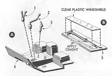
(A) Cement the transfer case shift 1, gear shift 2 and hand brake 3 into holes in floorboard 4 as shown above. (B) Apply cement to windshield frame 5 as indicated above and press clear plastic windshield in place.
