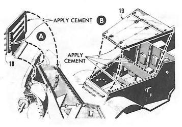
(A) Apply cement to back of grill 18 as indicated above and attach it to front of body. (B) Apply cement to top edge of dashboard, to top of ledges inside body and to front edge of hood 19. Fit hood in place and press it down tightly.
