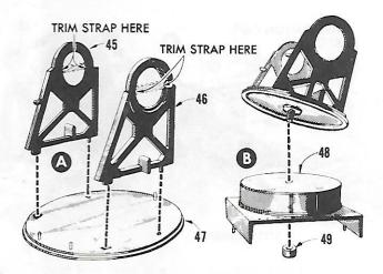
17 (A) Cut away straps from inside circles on frames 45 and 46. Cement left and right frames to turret 47 making certain that tabs fit into proper slots for correct positioning. (B) Insert post on turret through hole in turret mount 48. Carefully apply cement into hole in cap 49 and slip cap over post. Turret must revolve freely.
