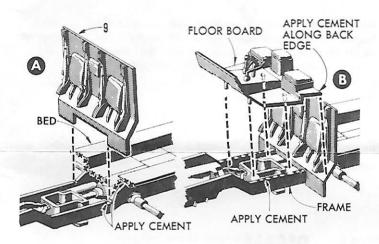
**3** (A) Apply cement to bed and frame as indicated. Attach cab back 9 making sure it is pressed tightly against bed. (B) Attach floorboard to frame as shown in illustration.
