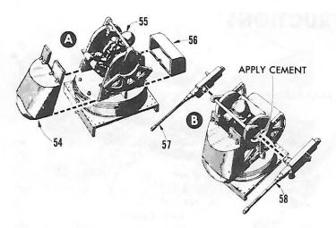
19 (A) Apply cement to gunner 55 and place in turret seat with helmet behind gun sight. Then attach front 54 and rear 56 shields to turret. (B) Apply cement to slots in right and left sectors and attach the .50 caliber machine guns 57 and 58.
