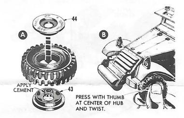
16 (A) Press wheel hubs 43 into tires. Apply cement sparingly to hub and slip wheel disc 44 into other side of tire as shown. (B) Place a small amount of petroleum jelly or grease into hole in each wheel hub. Press and twist wheels onto front axle past retaining ring until wheel spins freely. Be careful not to break axle.
