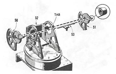
18 Insert seat 52 between frames as shown. Cement end of gun sight 53 having flat spot into "D" shaped hole in left sector 51. Gun sight and turret must be in exact position shown above. Apply cement to slot in sector and attach it to tab on seat. Next cement right sector 50 to seat tab and gun sight. Do not cement sectors to frames.
