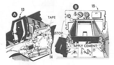
**5** (A) Insert both doors 13 and 14 into door openings in body sides. Do not cement them in place. Hold door in position with tape. (B) Apply small amounts of cement to areas shown in sketch and insert dashboard 15. Bottom of dashboard fits into "U" channel and top fits against stop shown. Do not get cement on door hinges or doors will not open.
