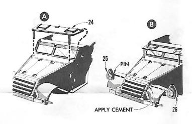
10 (A) Put a drop of cement into each hole in windshield frame and into two holes in hood and then fit windshield armor 24 in place. (B) Cement right 25 and left 26 headlights into holes in body sides. Push pin on headlight into hole until small stop button on back of pin hits body side.
