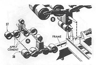
13 (A) Apply cement to ends of pins and to edges of inside bogie 37 in area shown above and join to outside bogie 38. Join other bogie halves in the same manner. (B) Turn model over on its back. Cement lineup pins on bogie between tapered pins on frame. Attach other bogie and allow cement to dry thoroughly before attaching track.
