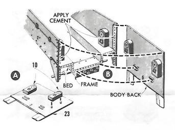
**9** (A) Cement two ammunition cases 10 to inside of body back 23 as shown in sketch A. (B) Put cement along ledges on body sides, on end of bed and frame. Attach body back to rear of body.
