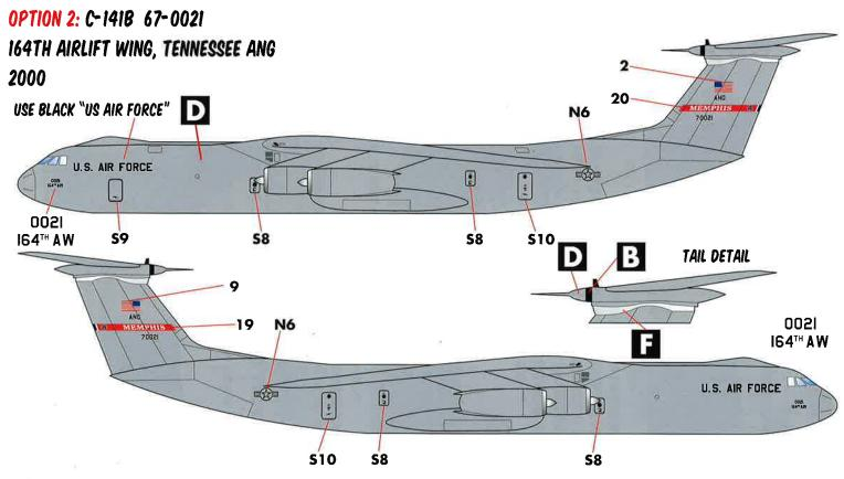
THESE DIAGRAMS SHOW THE TYPICAL STENCILLING AS SEEN ON USAF C-141B FLEET IN THE OVERALL AMC GRAY SCHEME AFTER THE 1990S.
